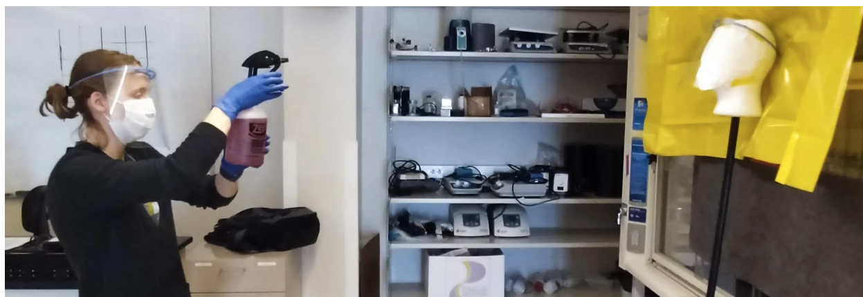
Bioengineering student Anne Lyons conducts a face shield spray test in the Bioscience 2 testing lab.
