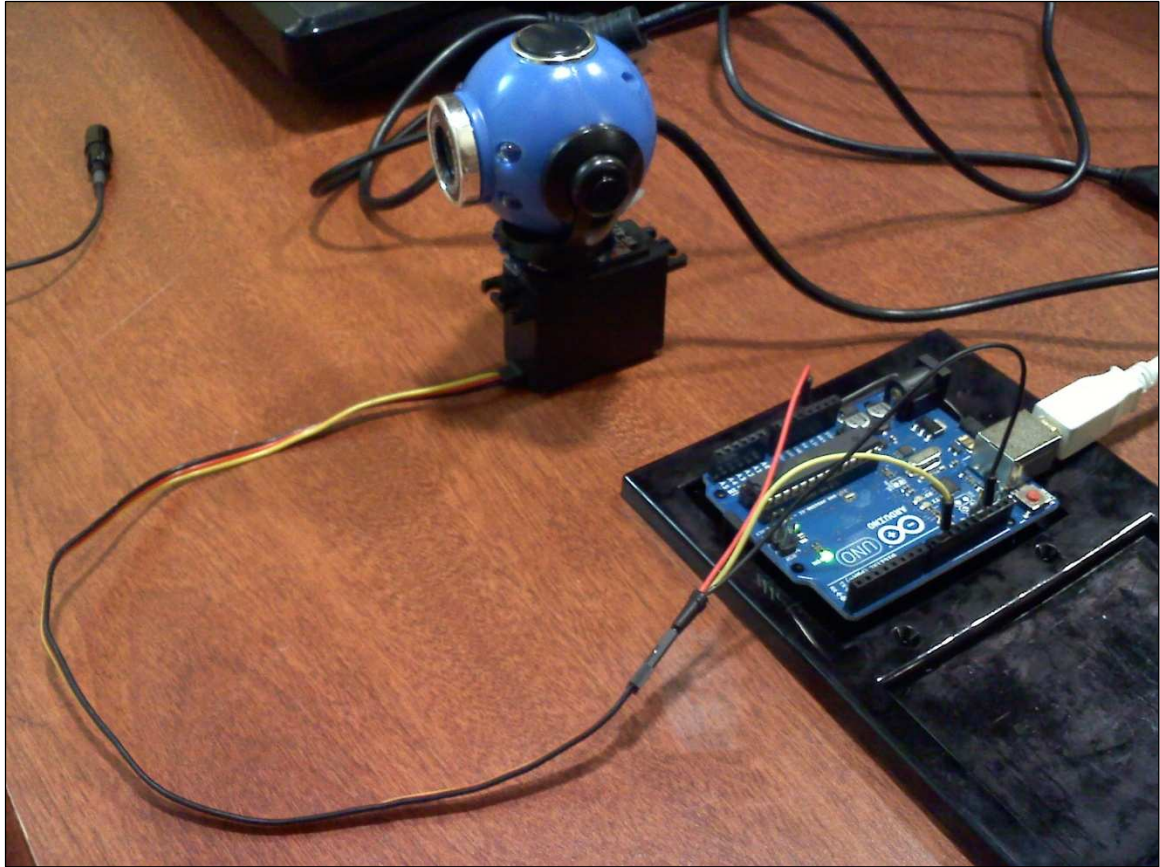
Figure 3.3 Gunshot Detection and Localization System, Arduino and Servo
