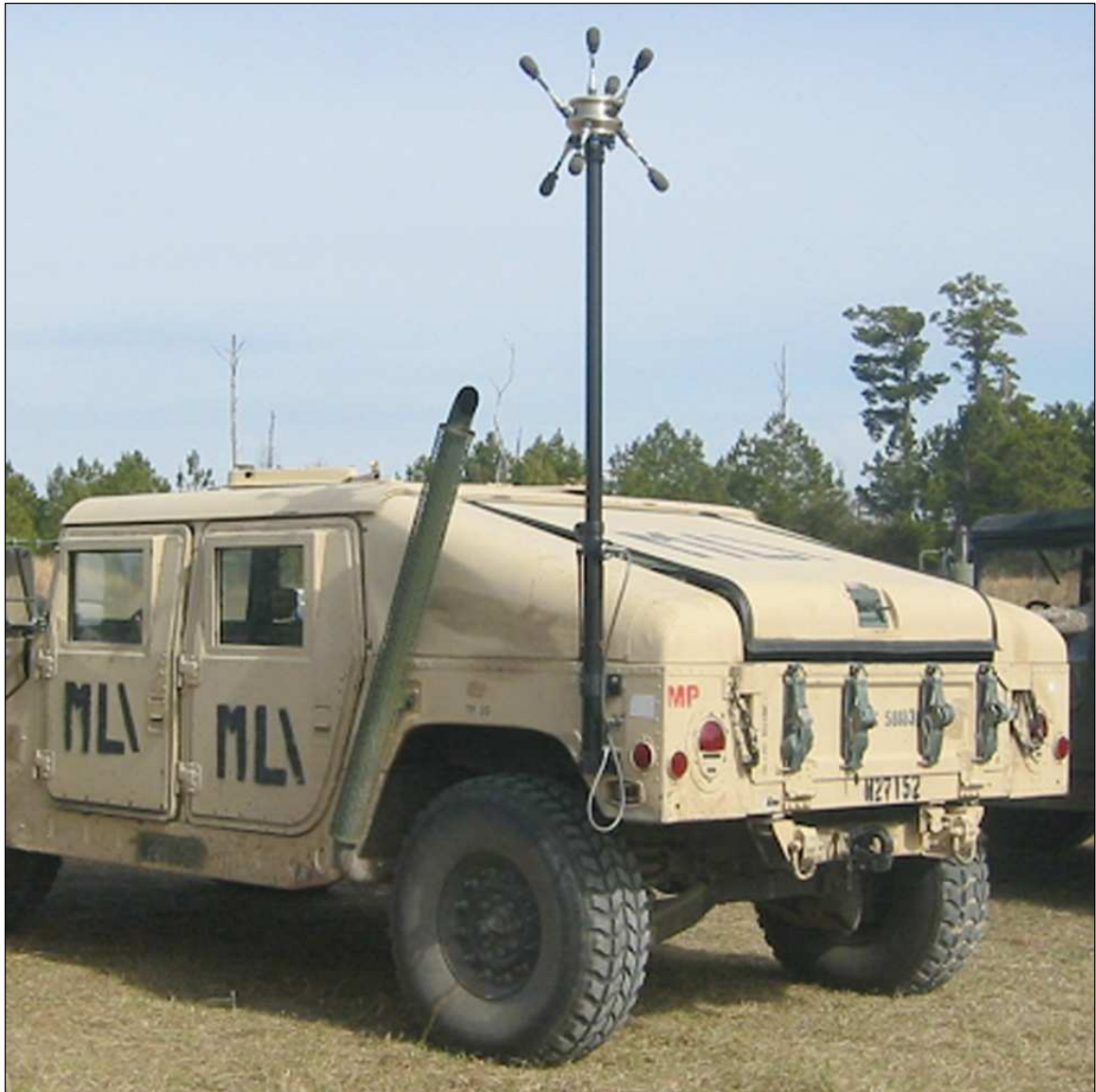
Figure 1.2 ‘Boomerang’ Gunshot Detection System, Outfitted to US Army Humvee
