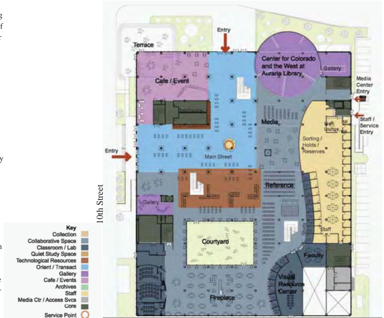
Figure 2.7: Proposed floor plan for first floor of Auraria Library
