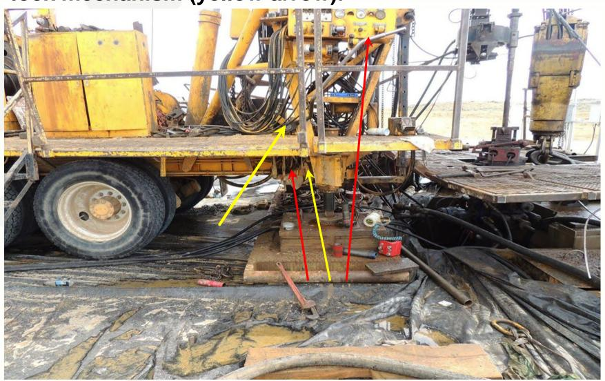
Brake linkage lock assembly with spring below operators station.
