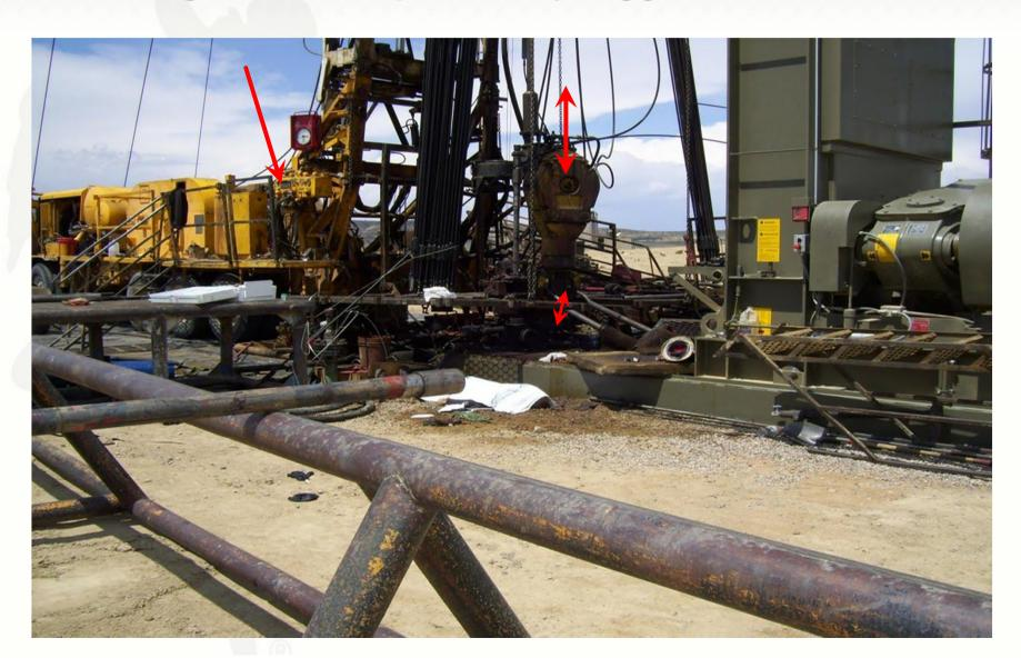
Operator station, brake handle (red arrow), linkage, lock mechanism (yellow arrow).
