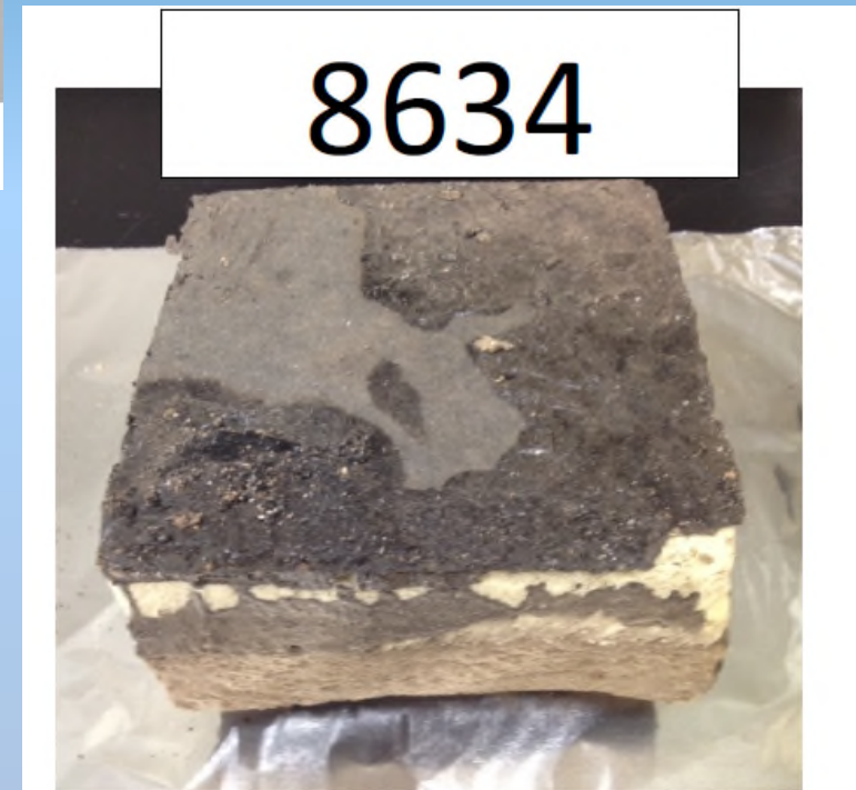
FIGURE 3. Roofing core sample #3 (HRG 8634) from AFA – Harmon Hall
